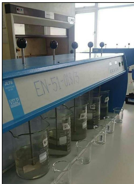
Image of a jar test by Jigchen L. Norbu is licensed under CC BY-SA 4.0
